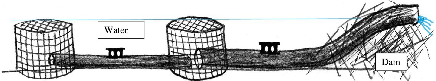
The “*Multi-Intake Leveler*” design is based on the highly successful Flexible Pond Leveler<sup>TM</sup> which has been successful in thousands of locations. This pipe system is intended specifically for use in narrow channels or where there is inadequate depth for a standard Flexible Pond Leveler. See diagram.
