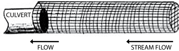
Diagram of a single cylindrical culvert protective fence (Beaver Solutions LLC, n.d.)
